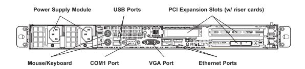
Note: the SC815TQ-560U chassis (5015M-U/5015M-NT) has only a single power supply module.
